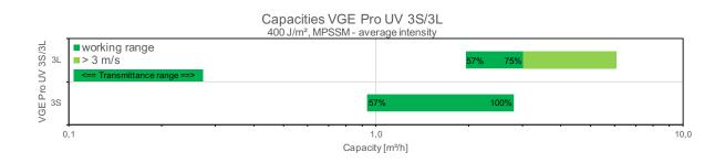
$An \,\, UV-C \,\, dose \,\, of \,\, 400 \,\, J/m^2 \,\, equals \,\, 40 \,\, mJ/cm^2 \,\, and \,\, the \,\, transmittance \,\, of \,\, the \,\, water \,\, is \,\, measured \,\, with \,\, UV-C \,\, light \,\, (254 \,\, nm) \,\, through \,\, 10 \,\, mm \,\, of \,\, water.$
