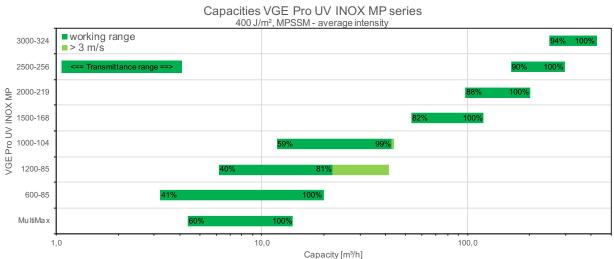
An UV-C dose of 400 J/m² equals 40 mJ/cm² and the transmittance of the water is measured with UV-C light (254 nm) through 10 mm of water.
