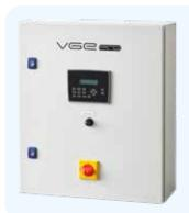
The Comfort control box is a complete control for the 600-85 to 3000-326 medium pressure units. The controller can optionally be equipped with a UV sensor to measure the UV-C intensity inside the treatment chamber. Besides that it is suitable for a temperature sensor. The temperature sensor monitors the temperature in the treatment chamber to avoid overheating. The display text on the controller is available with different languages.
